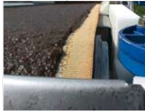
Separated particles transported to top of belt and drained to high matter content
